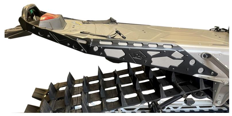
Note: Installation is for both length bumpers. (The 165 bumper is shown) The 155 rear bumper has one less rivet and one less bolt on each side.
