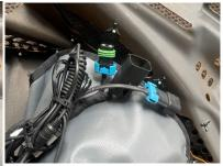
5. Lastly, you will need to install the upper rivet in the light bracket. There is a small flat space on the deck of the hood you will use to "AIM" your light in the correct direction along with the "up and down" movement where the light fastens to the bracket. Start the machine and "AIM" the light to get the upper hole location for where you want the light to shine. Drill the hole and install the rivet.
