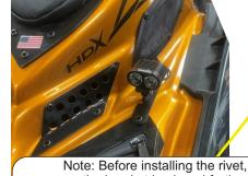
Note: Before installing the rivet, move the bracket back and forth until you get the direction of the light where you want it. Use the "up and down" movement on the bracket bolt in conjunction with the back and forth.
